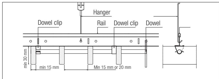
The distance between the dowels is 300 mm. The panels are connected to each other with a male/female dowel intersection which conceals the joint. A gap of 10 mm is formed between one panel and the adjacent panel.
